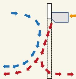
Air curtains are designed to be positioned above an entrance, providing a thermal curtain, which separates the outdoor and indoor environments. This historically has been produced by electrical heaters, however it is now possible to use a Toshiba heat pump system, with the added benefit of improved energy savings.
